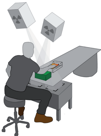
Figure 2. Dynamic radiostereometric setup during press test application. The patients were positioned with shoulder adduction, elbow flexion, and the approximately 90° pronated forearm resting in the horizontal plane with the hand flat on a custom-made weight platform logging the force (kg) gradually applied by the patients to their maximum, and released gradually, to no force, to induce dorso-volar directed translation of the ulnar head. A custom-made Raspberry Pi was used to timestamp dynamic radiostereometric image recordings (dRSA) (10 Hz), and further to record and relate the dRSA images and the force applied on the weight platform. The press test was performed during by 2 ceiling mounted X-ray tubes with 20°–20° tube position on the vertical plane, projecting on 2 digital image detectors (Canon CXDI-50RF) slotted beneath a uniplanar carbon box (Carbon box 24, Medis Specials, Leiden, The Netherlands). The source to image distance (SID) was 150 cm and the source to skin distance (SSD) was 100 cm. The exposures were 60kV, 630 mA, and 2.0 ms exposure time for acquiring a resolution of 2208 x 2688 pixels resolution (0.16 x 0.16 mm/pixel). Images were exported as multi-frame DICOM files.
