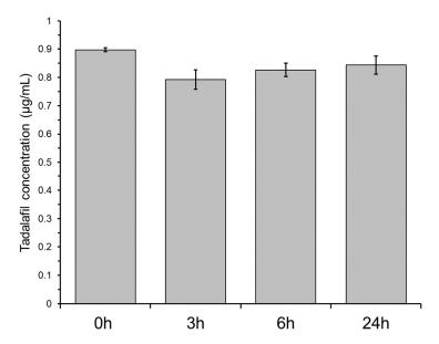
**Figure 4.** Non-specific adsorption of tadalafil to the plastic material of the two-compartment microplate system shown as the tadalafil concentration in the bottom-well after 3, 6 and 24 h incubation of a 0.9  $\mu$ g/mL tadalafil solution. '0 h' indicates the 'unincubated' (start) concentration. Data shown as mean  $\pm$  SD of six replicates.
