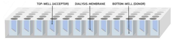
**Figure 1.** A schematic representation of the 96-well two-compartment microtiter plate.
