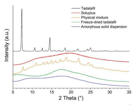
**Figure 3.** X-ray diffraction patterns of all formulations, tadalafil and Soluplus<sup>®</sup>.
