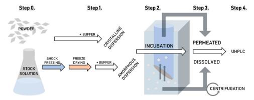
**Figure 2.** A flow-diagram of the high-throughput dissolution/permeation screening. Step 0. Formulation preparation, Step 1. Dispersion of the formulations, Step 2. Incubation of the two-compartment plate, Step 3. Sampling from the top-plate (acceptor) and bottom-plate (donor) and Step 4. Quantification of tadalafil by UHPLC.
