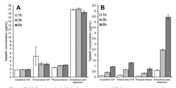
**Figure 6.** Tadalafil concentration in (**A**) the donor compartment and (**B**) the acceptor compartment after 1, 3 and 6 h of incubation when using different tadalafil formulations dispersed in 50 mM phosphate buffer as donor. The acceptor medium was 1% Vitamin E TPGS in 50 mM phosphate buffer. Data shown as mean  $\pm$  SD of four replicates.
