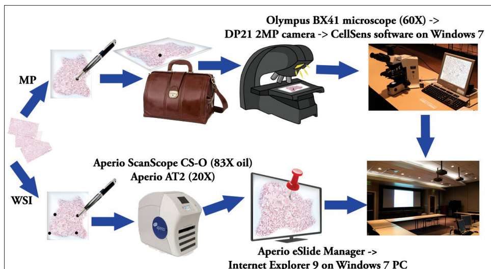
Figure 1: Schematic diagram illustrating workflow process for microscope projection (MP) and whole slide imaging (WSI) tumor board presentation methods. In MP, the slide is dotted to indicate fields of interest; it is then placed on a separate slide tray and physically transported to the conference room. The projection system consists of an Olympus BX41 microscope with a DP21 2 megapixel camera which is connected to a computer running CellSens software that captures the live video feed from the camera. With WSI, the fields of interest to be scanned are delineated using 4 dots. The slides are then scanned using an Aperio ScanScope CS-O scanner to scan at \times 83 magnification under oil immersion, or using the AT2 scanner at \times 20 magnification. The scanned slides are uploaded onto eSlide Manager and the fields to be displayed at treatment planning conferences are preannotated using the pinning function. At TB, eSlide Manager is opened via Internet Explorer. In both the MP and WSI methods, the computer screen is projected for viewing by attendees using a standard overhead VGA video projector
