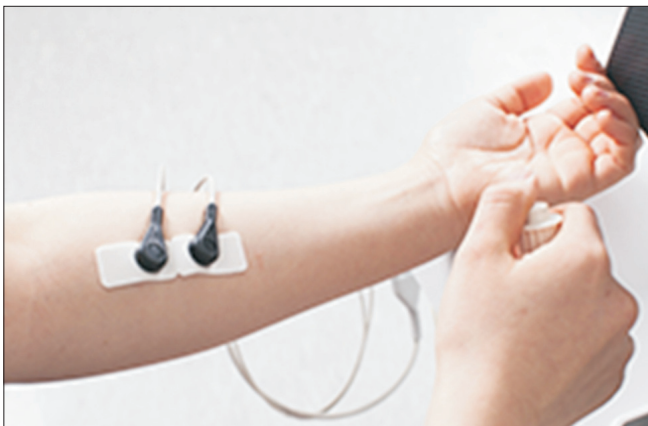
Fig. 1. Measuring position for quantitative assessment of pain perception. While in a comfortable seating position, the electrode patch is attached to the left anterior forearm and the stop switch is held in the right hand.
