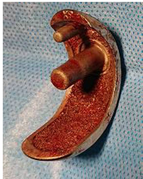
Fig. 3 Image of the retrieved femoral component. No bone is attached to the undersurface of the retrieved femoral component
