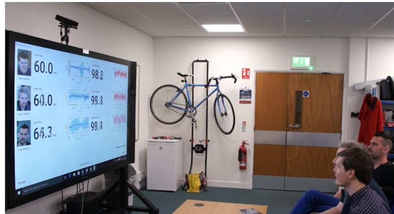
Figure 5. ARPOS live application demo image. The image shows peoples faces are identified on the left (monitor screen) where the heart rate is the blue line and blood oxygenation level is the red line plotted on the screen where the shaded regions represents the potential error.
