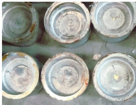
Figure 5. Scale-reduced parts of brake hub formed by rheological die forging.
