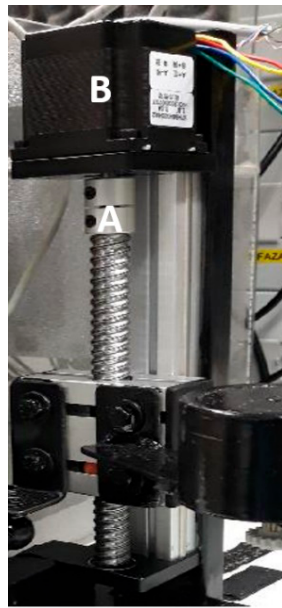
Figure 4. View of the distance adjustment circuit d (lens-observed component); A—worm gear; B—stepper motor to adjust the distance between the lens and the observed element.
