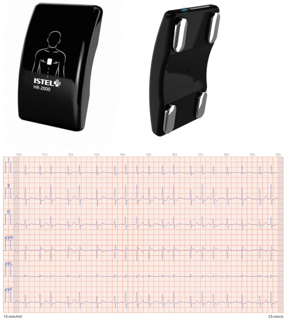
Fig. 1 The TTM recorder and the example of original recording with AF
