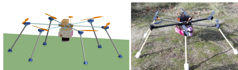
Figure 15. Drone and Sensorbox on the ground: CAD (left) and photograph, before takeoff (right).
