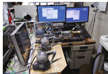
FIGURE 2: The L-shaped console consisting of the endoscope control system on the right (a) and the forceps control system in front (b): rotating handle (1), mini joystick (2), a PC monitor of an endoscope control system (3), a PC monitor of a forceps control system (4), a robot operation monitor (5), an endoscope monitor (6), two personal computers (PC) (7), two Geomagic Touch devices (8), and a master unit of the injection-needle catheter system (9).
