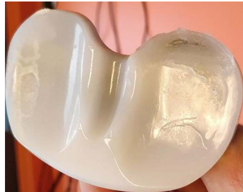
Figure 3: The tibial bearing showed wear mainly involving the posterolateral corner.
