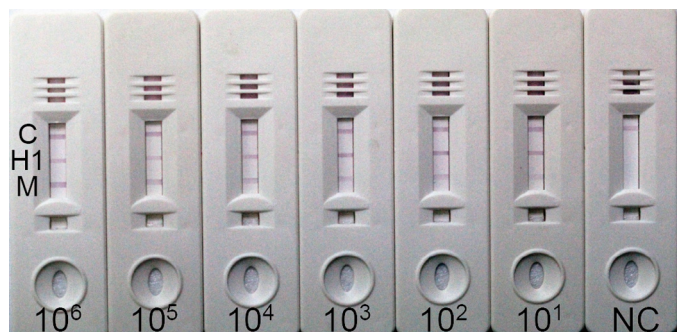
Fig. 6. LOD test of the multiplex RT-LAMP reaction targeting H1 and M genes by using influenza A H1N1 viral RNA templates ranging from 10^6 to 10 copies.
