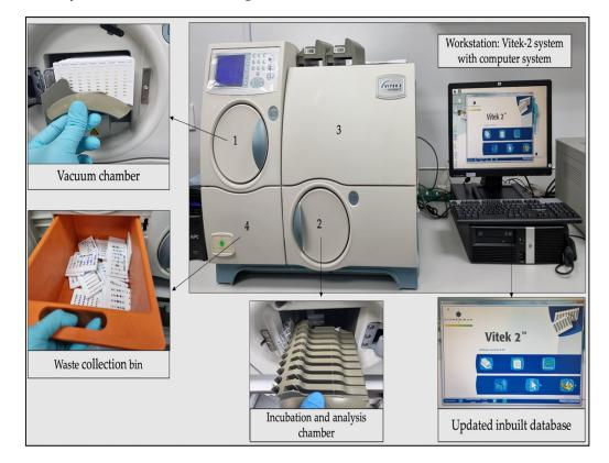
**Figure 2.** Workstation VITEK 2 system with computer system. Note: 1—fill door; 2—load door; 3—front user access door; 4—waste collection door.
