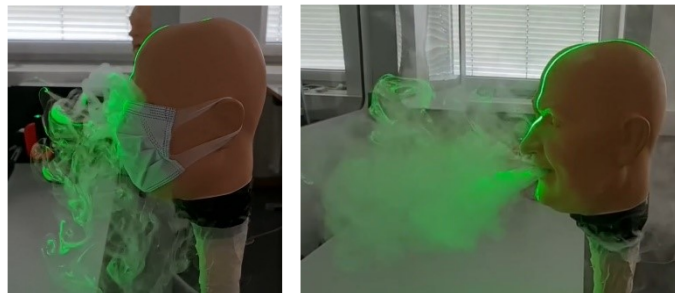
Figure 5: Flow visualization with and without face mask
