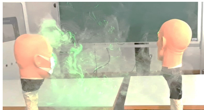
Figure 6: Even with everyday face masks, the aerosols spread into the room and reach the neighbour.
