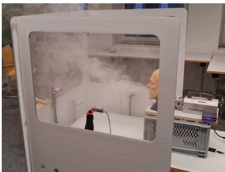
Figure 8: Reference using three-partition wall cabin with FlowMarker® and four Plantower PMS 7003 sensors
