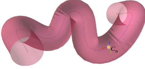
FIGURE 1: Schematic illustration of arbitrary point sampling on the centerline of the model. The black line represents the centerline of the model, and the surface of the model is red.
