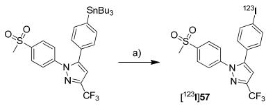
Reagents and conditions: (a) [123I]NaI in 0.01 M NaOH, NaI, CAT·3 H<sub>2</sub>O, 1 M HCl, H<sub>2</sub>O/EtOAc, r.t., 4 min.
