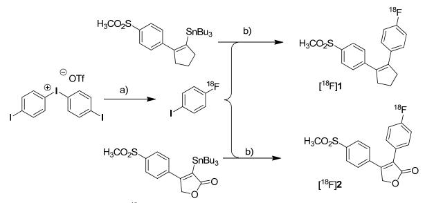
*Reagents and conditions*: (a) [<sup>18</sup>F]KF, K<sub>222</sub>, K<sub>2</sub>CO<sub>3</sub>, DMF, 120 °C; (b) different conditions, optimized:  $Pd_2(dba)_3/P(o-tolyl)_3/CuI$ , DMF-toluene, 65 °C, 20 min.
