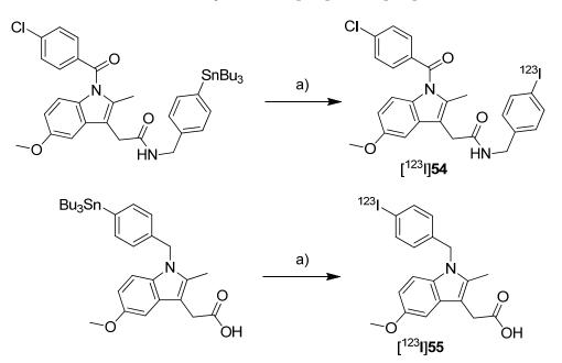
Reagents and conditions: (a) [1231]NaI in 0.01 M NaOH, NaI, CAT·3 H<sub>2</sub>O, 1 M HCl, H<sub>2</sub>O/EtOAc, r.t., 4 min.
