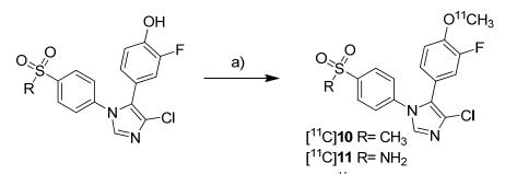
*Reagents and conditions*: (a) different conditions, optimized: [<sup>11</sup>C]CH<sub>3</sub>OTf, aq. NaOH, acetone, r.t. or 120 °C, 1 min.
