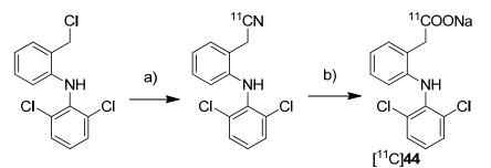
*Reagents and conditions*: (**a**) [<sup>11</sup>C]NaCN, DMSO, 110 °C, 10 min; (**b**) 10 M NaOH, 30% H<sub>2</sub>O<sub>2</sub>, DMSO/H<sub>2</sub>O, 135 °C, 10 min.
