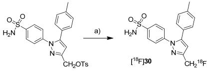
Reagents and conditions: (a) [18F]KF, K222, DMSO, microwave, 165 °C, 3 min.
