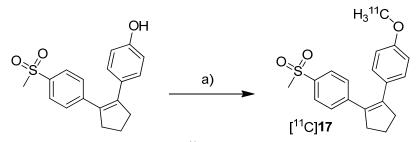
Reagents and conditions: (a) [<sup>11</sup>C]CH<sub>3</sub>I, NaOH, DMF, 60 °C, 3 min.
