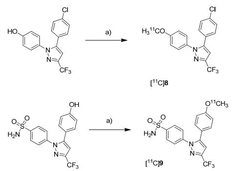
*Reagents and conditions*: (a) different conditions, optimized: [<sup>11</sup>C]CH<sub>3</sub>OTf, aq. NaOH, acetone, r.t., 2 min.
