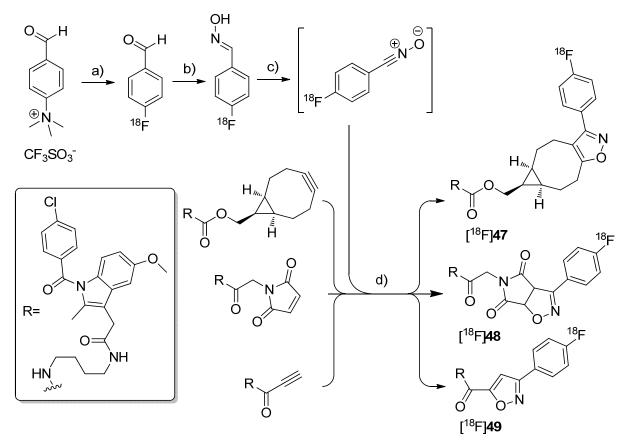
*Reagents and conditions*: (a)  $[{}^{18}F]KF,K_{222}$ , DMSO, 85 °C, 10 min; (b) NH<sub>2</sub>OH·HCl, 1 M NaOH, MeOH, 40 °C, 10 min; (c) PIFA in MeOH for  $[{}^{18}F]$ **47** and  $[{}^{18}F]$ **48**, BAIB in DMF for  $[{}^{18}F]$ **49**, 5–10 s; (d) MeOH, r.t. for  $[{}^{18}F]$ **47**, 40 °C for  $[{}^{18}F]$ **48**, 60 °C for  $[{}^{18}F]$ **49**, 10 min.
