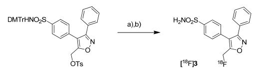
Reagents and conditions: (a) [18F]KF,K222, K2CO3, MeCN, 90 °C, 5 min; (b) 40% TCA in MeCN, 90 °C, 5 min.
