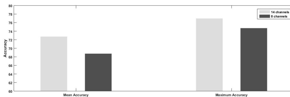
Figure 8. Comparison of mean and maximum classification accuracies achieved from subject-specific configuration of 8 and 14 electrodes, respectively.
