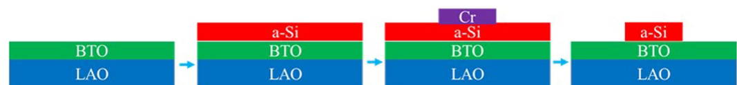
Figure 5. The fabrication process of the mid-IR waveguide sensor using Si-on-BTO platform. The epitaxial BTO film was grown on a (001) LAO substrate by PLD and then followed by a-Si thin film deposition through PECVD. Using photolithography and lift-off, the waveguide structure was first defined by a Cr mask, and then transferred to the a-Si layer by RIE.
