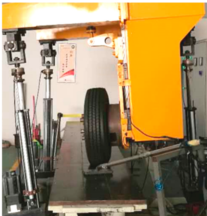
Figure 2. Bench test scenario of the tire mechanical properties.
