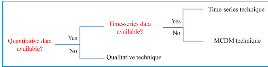
Figure 1. Applications of the three fuzzy techniques according to the availability of various types of data.
