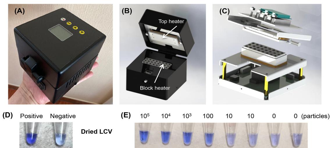
**Figure 5.** Block heater and dried reagents. (A), (B), and (C) outside, inside, and exploded views of our block heater. (D) Colorimetric detection of SARS-CoV-2 with the dried reaction mix and LCV dye. SARS-CoV-2 virions ( $10^3$ ) used in the positive control. (E) Colorimetric detection of SARS-CoV-2 with the dry LAMP reaction mixture in the presence of  $10^5$ ,  $10^4$ ,  $10^3$ , 100, 10, and 0 virions/reaction. These reactions were incubated with our custom-made block heater.
