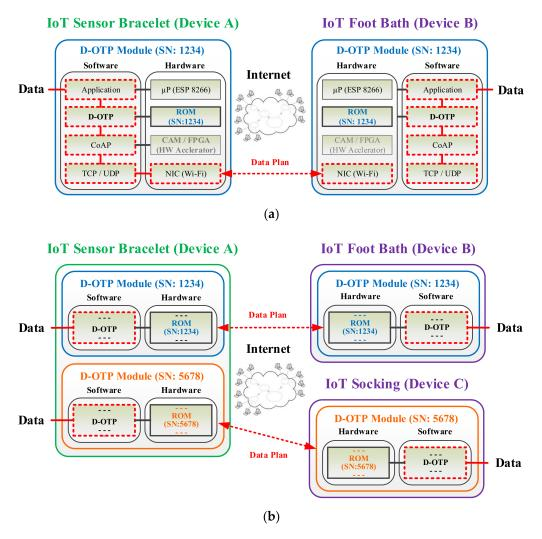
**Figure 6.** D-OTP architectures for directly transmitting data between (**a**) two or (**b**) three healthcare IoT devices.
