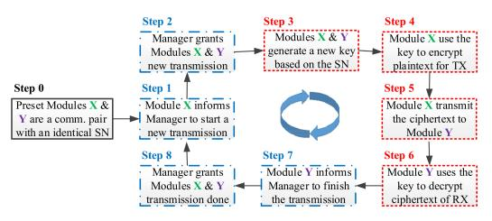
Figure 4. A D-OTP operation flow for activating the IoT secure transmission ecosystem.
