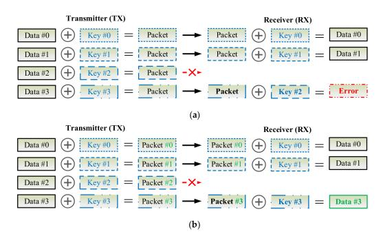
**Figure 10.** Scenarios where packets are transmitted through an unreliable transport (**a**) cause a key synchronization problem or (**b**) are patched by a basic solution to skip the key of the lost packet.
