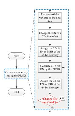
Figure 9. Execution flowchart of generating a new key in CoAP io.
