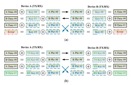
**Figure 11.** Scenarios where packets transmitted simultaneously from both devices (**a**) cause a key synchronization problem or (**b**) are patched by a basic solution to separate the keys used for TX and RX.
