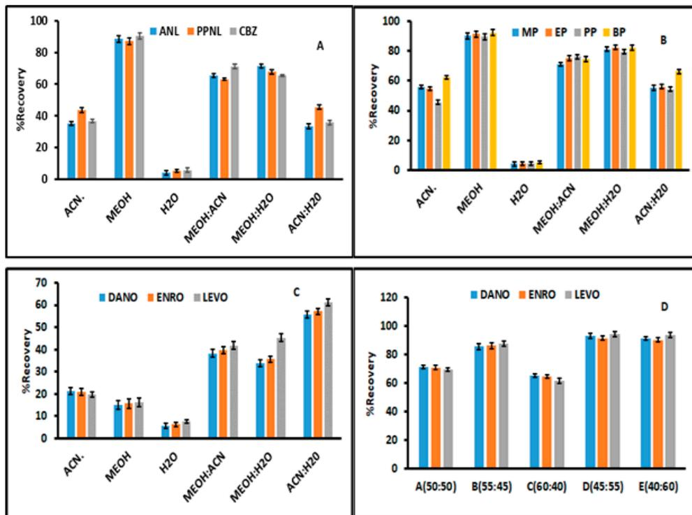
**Figure 1.** Recoveries of different elution volumes using different solvents for residual analytes. (A) Anticonvulsants and  $\beta$ -blockers (atenolol (ANL), propranolol hydrochloride (PPNL) and carbamazepine (CBZ)), (B) parabens (methylparaben (MP), ethylparaben (EP), propylparaben (PP) and butylparaben (BP)), (C,D) fluoroquinolones (danofloxacin (DANO), enrofloxacin (ENRO), levofloxacin (LEVO)).
