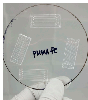
Figure 2. Bonded PMMA microchips on PSC-PC film.
