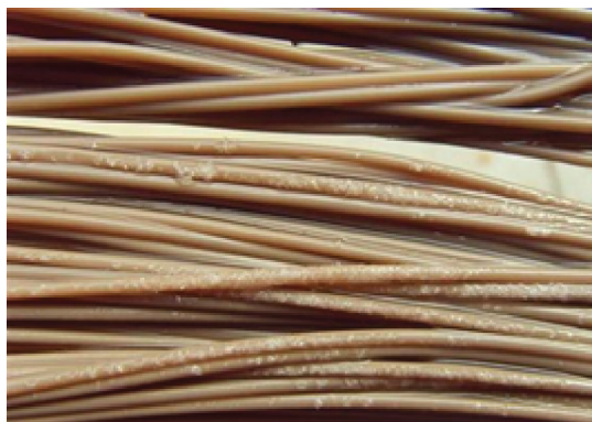
FIGURE 7: The photograph of NaCl crystallization on the surface of the membrane.
