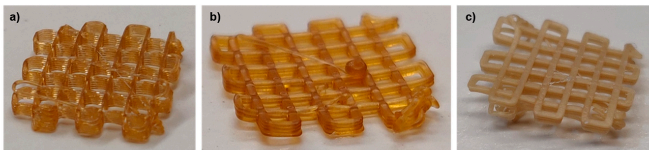
Figure 4. Photos of 3D-printed grids of 10 mm × 10 mm. (a) SIBS-B15; (b) SIBS-B15 mixed with TA (5 wt %); (c) SIBS-B15 mixed with TA (5 wt %) after the drug release. Height of the printed specimen is approx. 5 mm.
