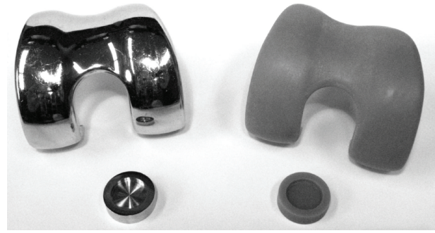
FIGURE 1: The Columbus CR prosthesis (Aesculap AG, Tuttlingen, Germany; top) and the test pieces (bottom) for the friction test made of the standard material (CoCr29Mo6) on the left and the rapid prototype material (RGD840) on the right side.
