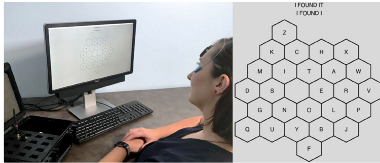
Figure 4. Example experimental setup and personalized keyboard. An individual navigates their personalized keyboard to spell “I FOUND IT” using the sEMG/IMU access method.
