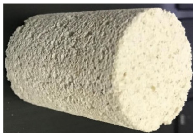
Figure 4. Aerated concrete core sample.
