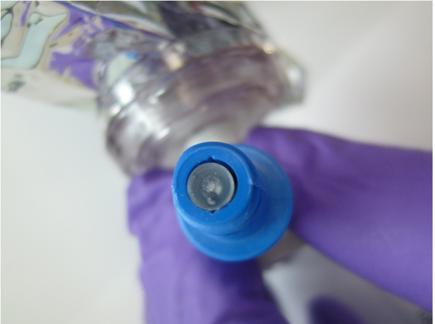
Fig 4. Liquid droplets observed on the membrane of ChemoClave CSTD following task 2.
