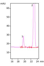
Figure 1. HPLC profile of the *n*-hexane extract of irradiated *P. ostreatus* powder. 1. Vitamin D<sub>2</sub>; 2. ergosterol.
