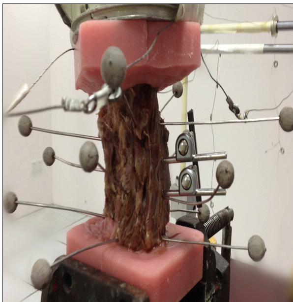
Figure 2. The test method for the range of motion of the cervical vertebrae under a 2.50-Nm force moment load.
