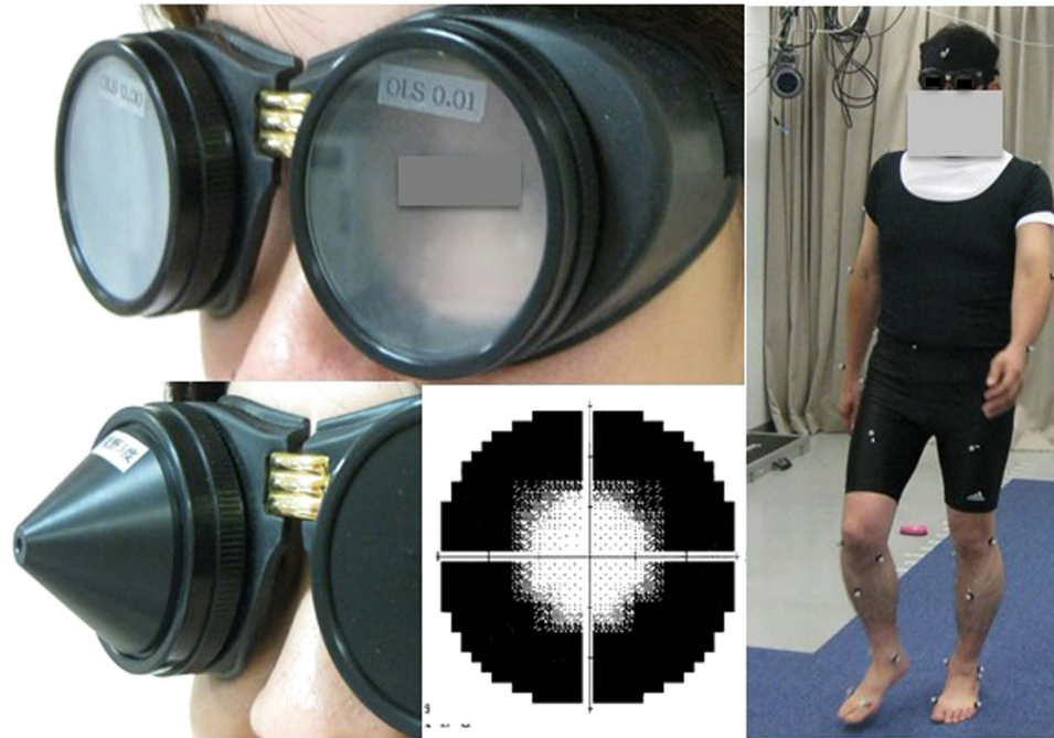
Figure 1. Simulation goggles and simulated visual field. “Simulated patients” wore goggles (top left) to simulate reduced visual function to the vision of 20/600. Representative results of visual field analysis (Humphrey Field Analyzer 30-2 program; Carl Zeiss, Jena, Germany) with goggles restricting the visual field to 3° show a successful simulation effect (bottom left and center). Motion analyses were performed using a motion capture system comprising eight cameras and a force plate (right).
