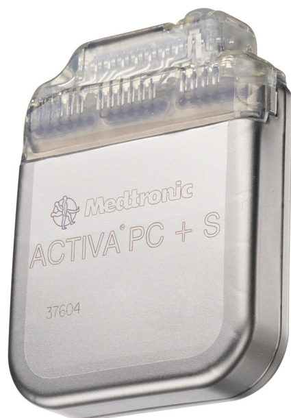
Fig. 3 The Activa® PC+S deep brain neurostimulator (Medtronic, Minneapolis, MN, USA). Reprinted with the permission of Medtronic, Inc. © 2013
