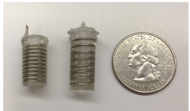
FIGURE 5. The manufactured antenna sensors with PDMS packaging.
