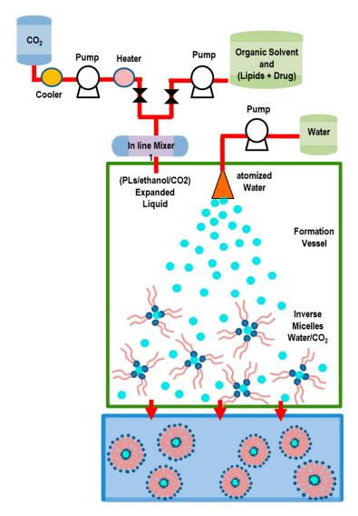
**Figure 12.** SuperLip method and mechanism of liposome formation. A high-pressure vessel is filled with an expanded liquid mixture (formed by PLs/ethanol/CO<sub>2</sub> containing drugs). Water droplets are produced by atomization inside a high-pressure vessel. These droplets are rapidly surrounded by a lipid layer, forming a  $w/CO_2$  emulsion (inverted micelle). Finally, liposomes (w/w emulsion) are formed when they fall in the water pool located at the bottom of the vessel.
