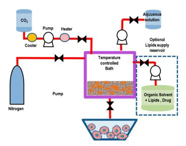
**Figure 13.** Schematic representation of the DELOS method. The lipids dissolved in organic solvent contained in a vessel at desired temperature and pressure, are mixed with SC-CO<sub>2</sub> (used as a cosolvent to the organic solvent). Then, the mixture (depressurized at 35–55 bar) is expanded into CO<sub>2</sub>, and injected through a nozzle into in a vessel containing water bath and active drugs, where the liposomes are formed.
