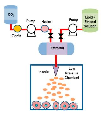
**Figure 11.** Schematic representation of the RESS method for liposome preparation. Initially, lipids are dissolved in supercritical  $CO_2$  and ethanol (5–10% of v/v) within an extractor. The resulting solution is depressurized through a heated nozzle in a low-pressure chamber. Finally, the formation of particles is generated, due to the supersaturation.
