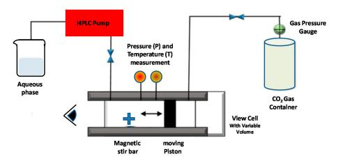
**Figure 9.** Schematic representation of the apparatus used in the supercritical reverse-phase evaporation method [109].
