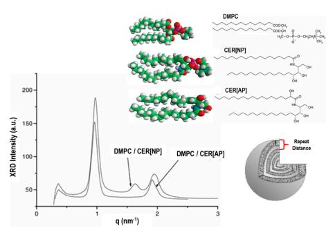
**Figure 17.** X-ray diffraction patterns for the mixed lipid system composed of DMPC/ $\alpha$ -hydroxy-N-stearoyl phytosphingosine CER[AP] and of DMPC/N-stearoyl phytosphingosine CER[NP] multilamellar vesicles (MLVs) at the temperature of T = 30 °C Adapted by permission from Springer Nature: [156] (Appl. Phys. A) by Kiselev et al., Copyright 2013.
