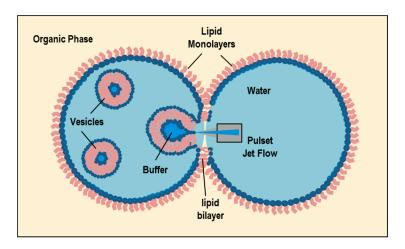
**Figure 15.** Schematic representation of the pulsed jet flow method. The lipids initially dissolved in the organic phase self-assemble (at the oil–water interface) as monolayers. The periodic pulses of a fluid jet (of a buffer) is directed at the interface of two nearby W/O microemulsions, and favors the formation of giant unilamellar vesicles [133].
