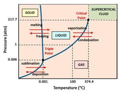
Figure 8. Phase diagram of carbon dioxide.
