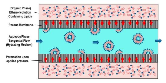
Figure 16. Liposome formation process in the membrane contactor method.
