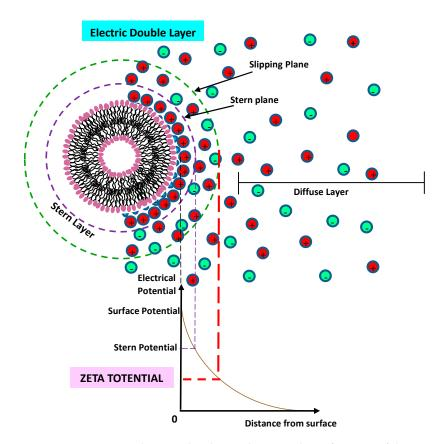
**Figure 19.** Diagram indicating the electrical potential as a function of the ionic concentration (and distance from the charged surface) of a liposome suspended in a dispersion medium.
