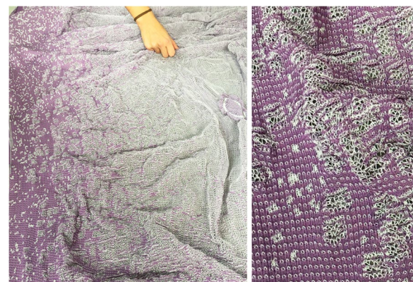
Fig. 4 Grading strategy for knitted membranes and their simulation. Knitted membrane can be simulated as a cablenet-like quad-based mesh, as it represents the UV-directionality of the knit and the pliability of the surface under the loads. For representing graded properties, each mesh segments is assigned a variagated stiffness value, which results in differentiated contraction (or expansion) of the digital mesh and represents graded property of the membrane surface. CITA 2022
