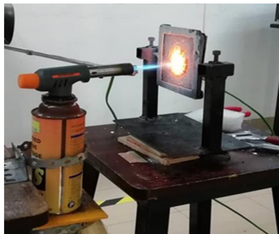
Figure 6. Setup for the fire retardant test.
