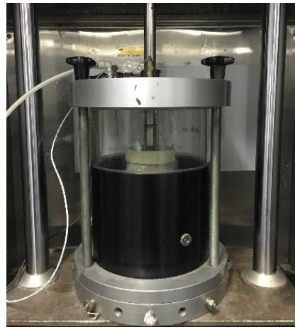
Figure 3. Equipment of triaxial tests.
