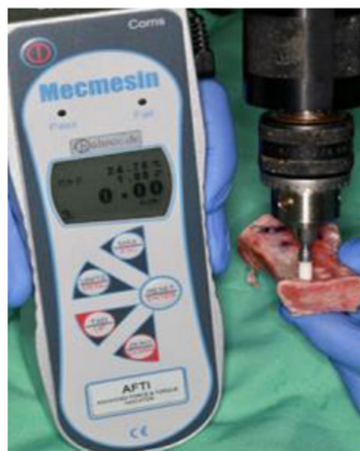
Fig. 3 Torque measurement conducted using the AFTI force and torque indicator
