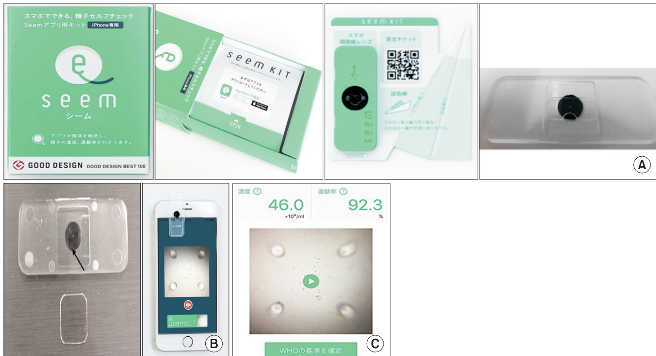
Fig. 1. Devices and components for the smartphone-based computer-assisted semen analysis (CASA) system. (A) Photo of the SEEM ® kit with instructions for use, sperm analysis device, semen transfer device, QR code sheet to download the application for operating, and disposable built-in counting chamber with objective lens and cover glass. (B) The technique for observing the semen sample using smartphone-based CASA. After a drop of semen (black arrow) is placed under the covered glass of the built-in sperm-counting chamber, the black-colored lens portion of the chamber is put on the front lens of the smartphone. (C) Sample screenshot of the captured test results of a semen sample with concentration and motility.
