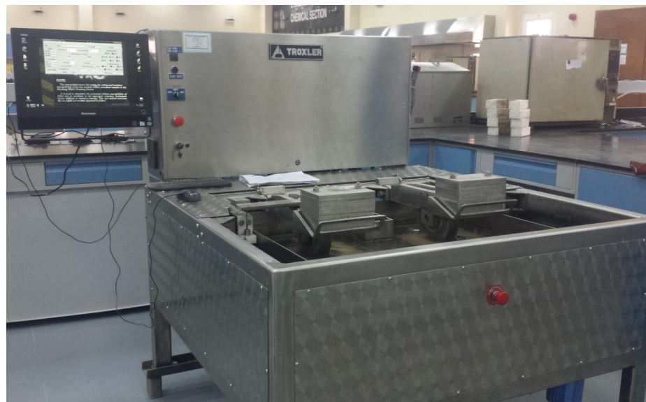
Figure 6. The Hamburg wheel tracker.
