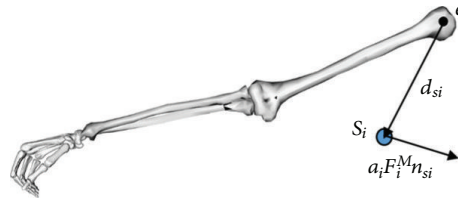
FIGURE 8: Free body diagram of the humerus that considers muscle forces.
