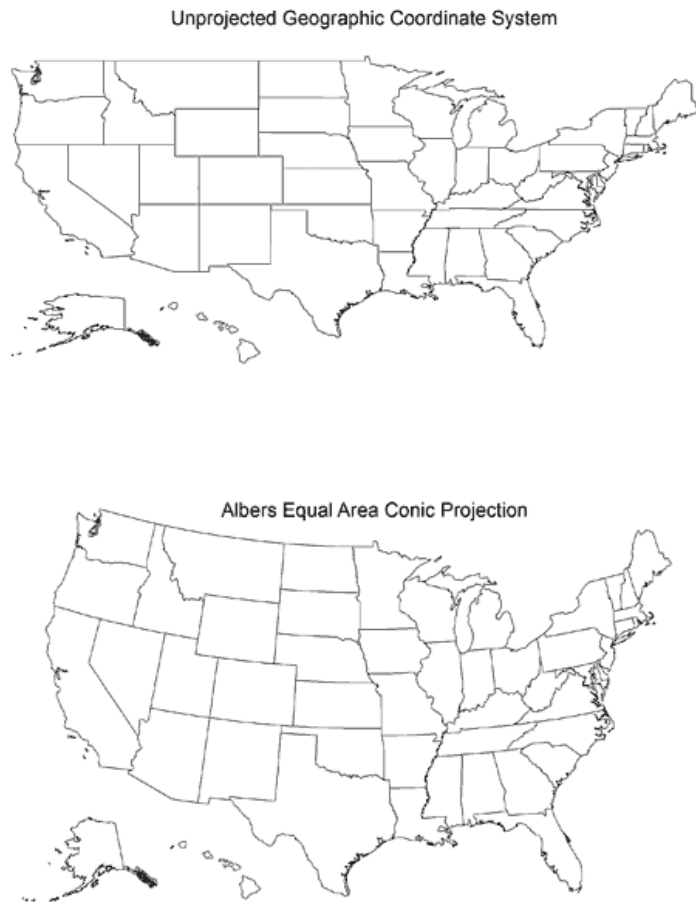
Figure. Two drawings of a US map. The top map uses unprojected geographic coordinates; the bottom map uses the Albers Equal Area Conic projected coordinates.
