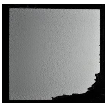
Figure 7. Photograph of a high-resolution scintillator screen consisting of a ^{10}\text{B}_2\text{O}_3 neutron converter in a 1:1 ( ^{10}\text{B} :ZnS) mix ratio with a ZnS:Cu scintillator with 4.7 \mu\text{m} median particle size.
