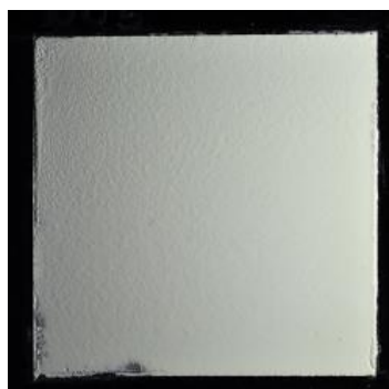
Figure 6. Photograph of a double-wedged scintillator screen consisting of a boron carbide converter ( ^{10}\text{B}_4\text{C} ) and a ZnS:Cu scintillator with 11.5 \mu\text{m} median particle size.
