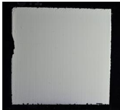
Figure 5. Photograph of a wedged scintillator screen with an oblique light applied to enhance the appearance of the surface texture. The screen shown is a ^{10}\text{B}_2\text{O}_3 neutron converter in a 1:1 ( ^{10}\text{B} :ZnS) mix ratio with a ZnS:Cu scintillator with 11.5 \mu\text{m} median particle size.
