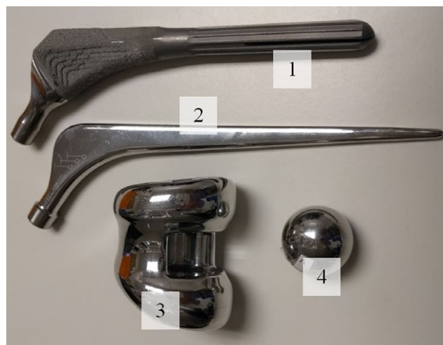
FIG. 1. Different prosthetic pieces used. (1) titanium, (2) stainless steel, (3) CoCrMo, (4) Vitallium™.
