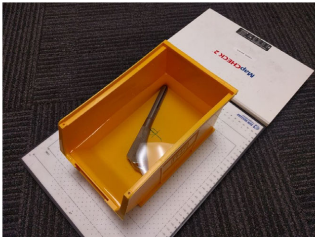
FIG. 2. Placement of prosthetic in water bath on top of MapCheck ® device.
