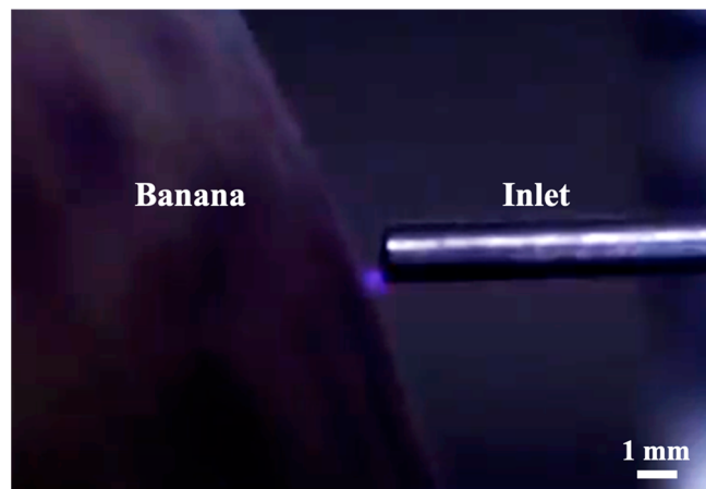
Figure 2. Photograph of a banana placed in front of the mass spectrometer applied with -4.5 kV during MS ionization.
