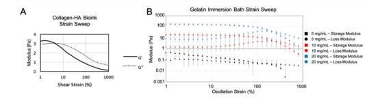
**Figure 3.** Rheological assessment of collagen–HA bioink versus gelatin bath solution. Storage and loss moduli data resulting from strain sweep tests from 1% to 1000% shear strain ( $\gamma$ ) for (**A**) the collagen–HA bioink and (**B**) gelatin solutions (5, 10, and 20 mg/mL).
