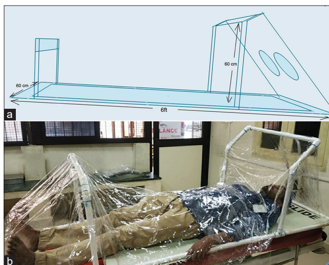
Figure 2: (a) Schematic diagram of pipe-framed patient coverall, (b) pipe-framed patient coverall used for patient shifting
